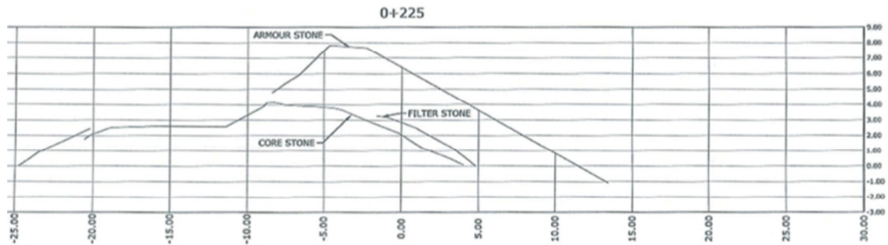
Figure As-Built Elevations [6]
